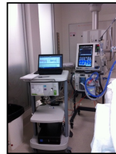
Figure 1. Quark RMR™ device for measuring metabolic rate
